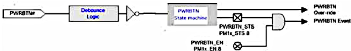
Fig. 4.8: Fixed Power Button Logic
