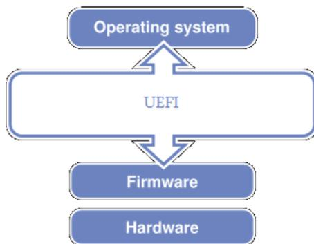
In addition to the services UEFI defines, there are various protocols/APIs to access various hardware and the boot devices in the system. The UEFI spec also defines a generic framework and can be adapted to any type of bus or device, knowing that computer hardware is constantly evolving. Visit <http://www.uefi.org> for more information on the UEFI Forum that controls the UEFI specifications or to download the UEFI specifications.
